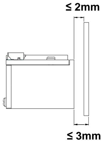
If the window is required to be in a tilted position, the above distance requirements should be met and tilt angle should ensure no reflections back into the lens.
